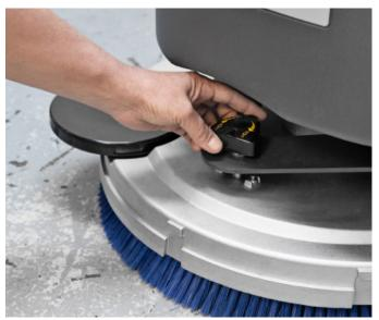
6. Adjust (if needed) the brush deck to have the correct machine directionality
