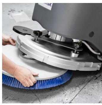
**1** Check if the brush are correctly installed and not worn out.
