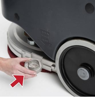
**2** Check if the solution filter is cleaned.
