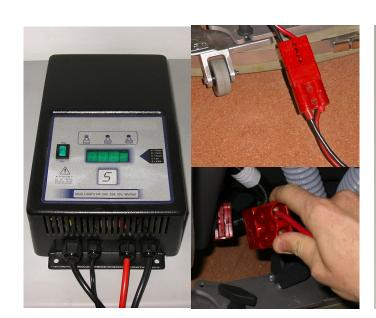
1a. Switch off charger by unplug charger cable from red battery plug. Reconnect the red battery plug to the machine.
