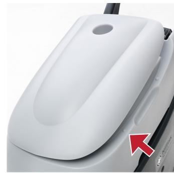
**4** Close the recovery tank cover properly and/or verify the gasket wear.
