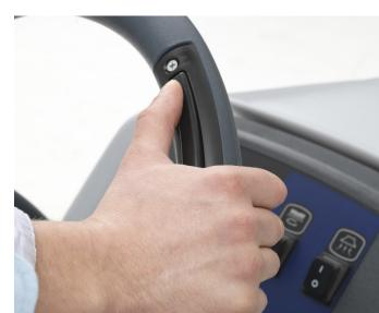
9. Press the handle switch to engage the brush and run the machine
