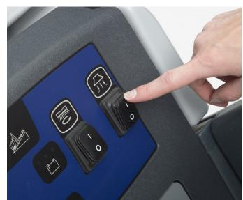
8. Switch on the brush and vac motors to activate the machine
