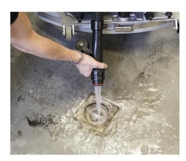
10. At the end of the work. Empty the recovery tank with the hose. Then empty the solution tank with the trasparent hose
