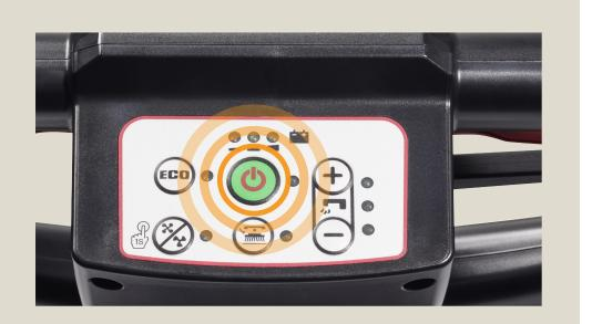
Turn on the machine and verify there is enough battery power to complete the work. Charge batteries if required.
