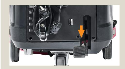
Lift the deck by pressing the pedal
