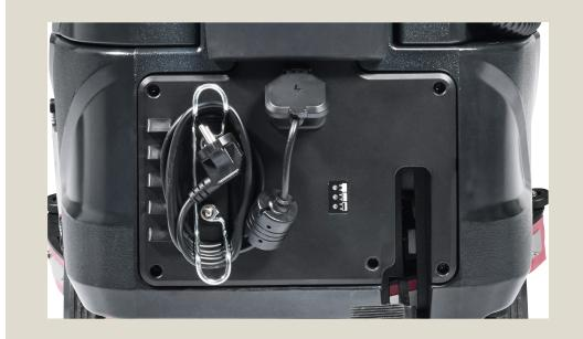
**Daily:** Charge the batteries: Connect the battery charger cable to the electrical socket. Light turns red when charging and green when the charging is complete.
