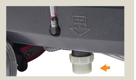
**Weekly:** Inspect the solution filter and clean if required.
