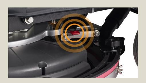
Lift the squeegee up by hand until it locks in up position and turn suction off for double scrubbing. To go back to working mode, use the red lever to release the squeegee. and turn suction on again.
